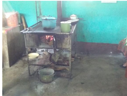
Fig. 10 - Fuel efficient stove
