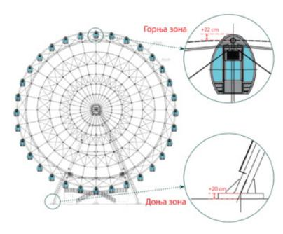
**Picture no 21:** Extract from the graphic part of the conceptual design for the construction of a Ferris wheel. (Front view)
