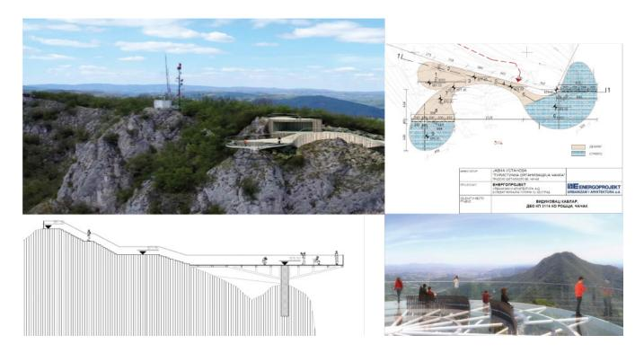
**Picture no. 18:** Excerpt from the architecture project, which is an integral part of conceptual solution number 3010/22 IDR-1 for the construction of the observation deck on Kablar
