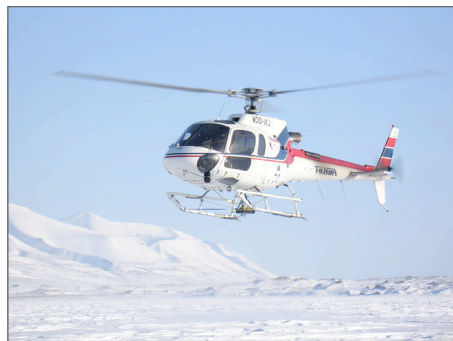
GPR Mounted Under Helicopter, MMS TAR 569
