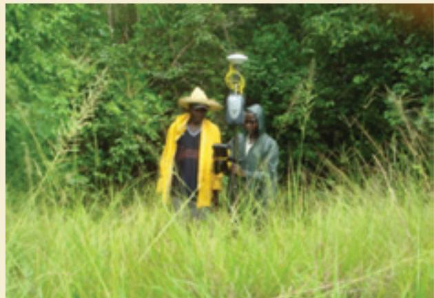
Figure 22. The RTK system, composed of (a) setting a base station by static surveying (left), and (b) RTK mode with both base (left) and rover (right) working together (Kimeu & Machano, 2011).
