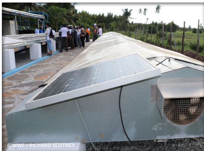
Newly installed solar drying technology capable of drying both seafood and terrestrially grown agriculture products like casava.
