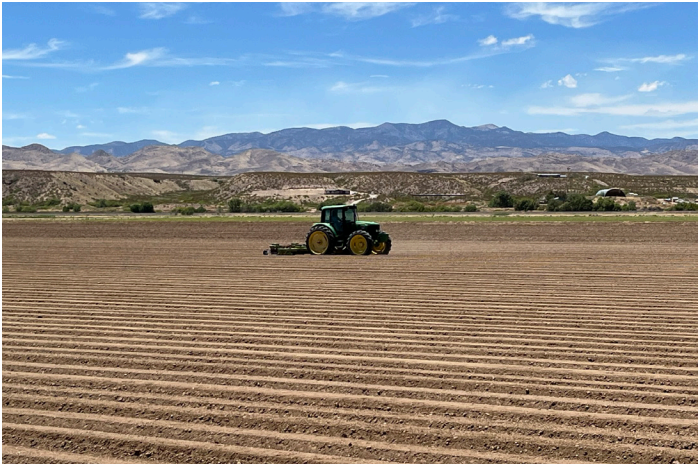
Laser leveling and GPS guided tractors reduce irrigation losses in the Middle Rio Grande Conservancy District, by Enrique Prunes.
