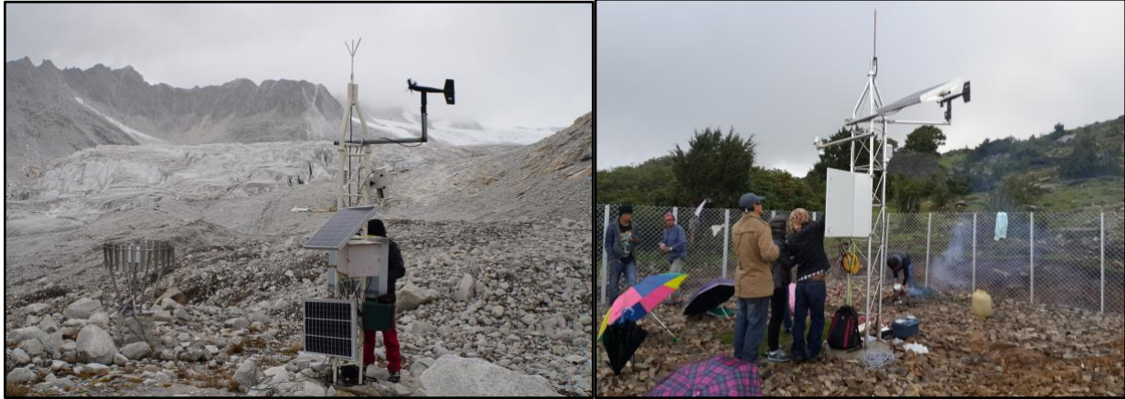
Figure 3: Sample pictures of AWS stations to be set up (Left: AWS at Thana Glacier, Right: AWS at Chelela)
